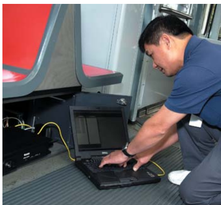
A Muni employee downloads video data from a 5308 MDVR mounted in a light rail vehicle
