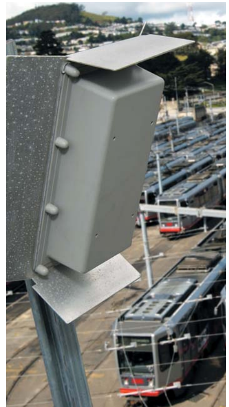
Wireless antennas mounted in Muni's light rail vehicle yard transmit video data from onboard March Networks 5308 MDVRs to a central server.
