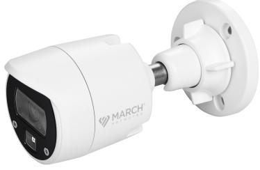
For customers who need a cost-effective compact camera, the **EL2 IR Bullet** from March Networks<sup>®</sup> integrates active IR illumination, and 2MP resolution to deliver high-quality images in a variety of lighting conditions. This essential camera is rated for indoor and outdoor use with a housing designed to be weather-proof (IP66 and IP67) and vandalresistant (IK10).
