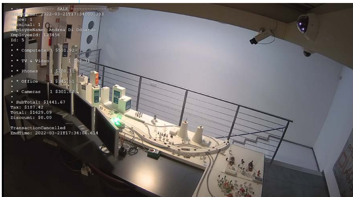
Figure 6: Associating a camera to a text channel — it's possible on the Client side to overlay the received data on the video stream.
