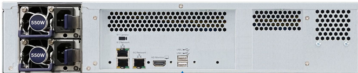
Two USB 2.0 Ports on back (USB 2 and USB 3)
