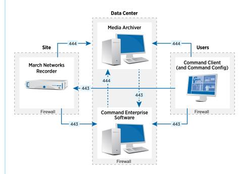
This approach will require each recorder to have local port 443 translated to a published address using the Network tab settings in March Networks Command Client. This setting is available once you are locally connected to the recorder with Command Client.
