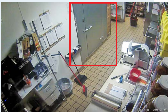
The "Abandoned Object" analytic triggers an alarm when an object is added to a designated area. In this instance above, a new object would block the door.
