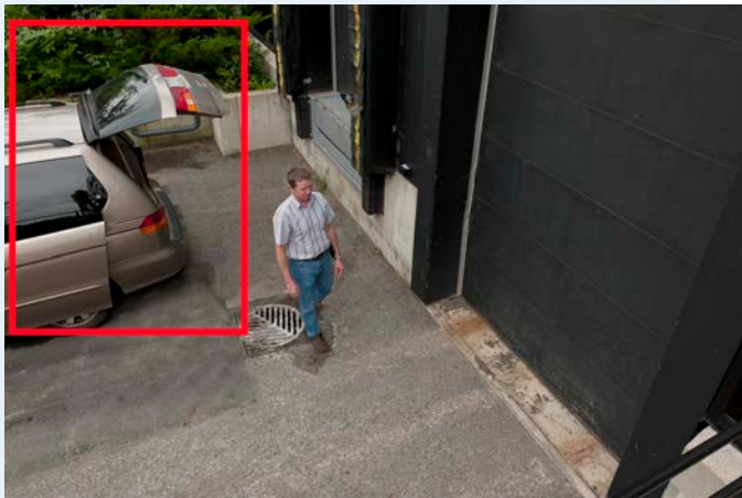
The "Loitering Detection" analytic triggers an alarm when a person or object lingers in a particular area for too long.
