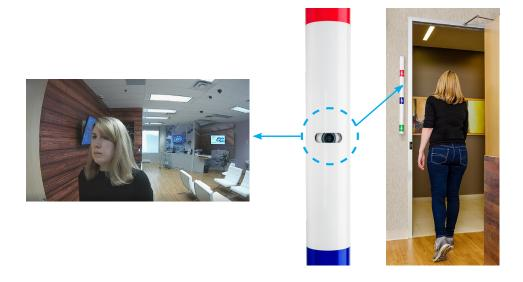
Install in a height strip housing for crystal-clear face shots at eye level
