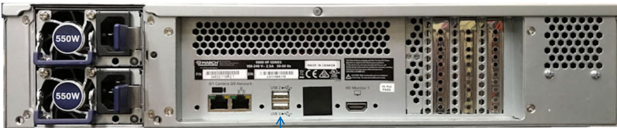
Two USB 2.0 Ports on back of 2U model (USB 2 and USB 3)
