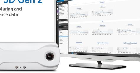
The **Brickstream**<sup>®</sup> **3D Analytics Sensor** captures and analyzes data on people counts, queue lengths/ wait times, presence detection, and service arrivals/ service times. These valuable metrics can reveal meaningful and actionable information on employee and customer behavior to improve customer service, optimize labor, increase revenues, and improve overall customer experience. The Gen 2 sensor features increased coverage, integrated mounting, and backward compatibility.
