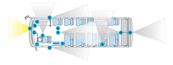
NOTES: <sup>1</sup> March Networks' mobile video surveillance equipment integrates with other onboard vehicle systems through a J1939/CANBus interface.
