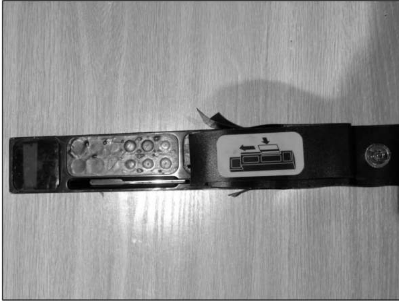
Figure 12 ATM Door Opener Skimmer Placed Over Legitimate Door Opener
