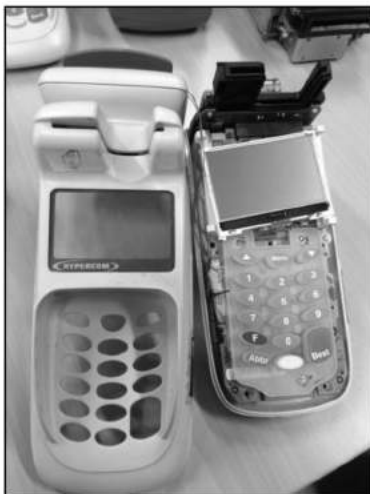
Figure 17 Thales POS Terminal with Cover Removed
